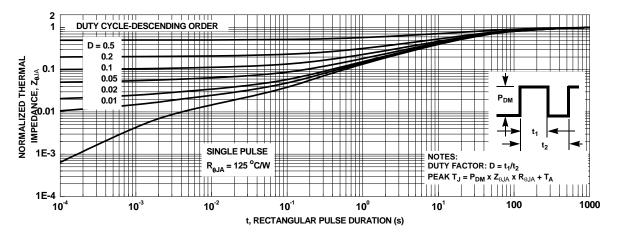
Figure 13. Junction-to-Ambient Transient Thermal Response Curve
