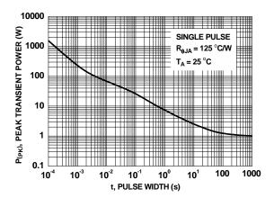
Figure 12. Single Pulse Maximum Power Dissipation
