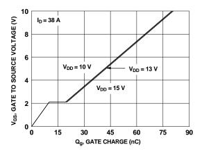
Figure 7. Gate Charge Characteristics
