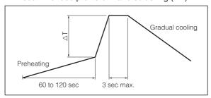
$\triangle T$ : Allowable temperature difference  $\triangle T \le 150$  °C
