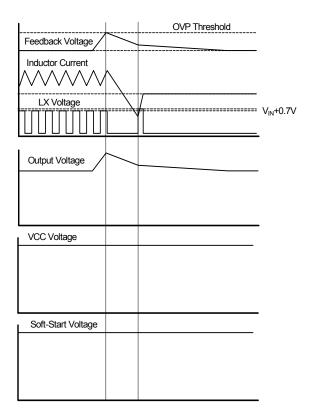
Figure 6. OVP Timing Chart of AOZ2151PQI-05
