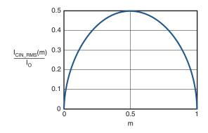
Figure 7. I<sub>CIN</sub> vs. Voltage Conversion Ratio
