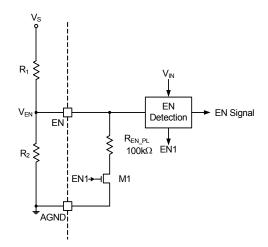
Figure 2. Enable Internal Circuit of AOZ2151PQI-05
