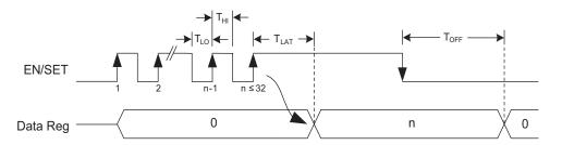
Figure 1: S2Cwire Timing Diagram.
