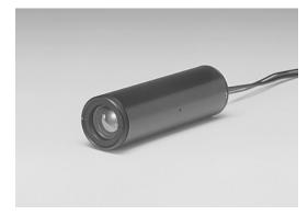
The H7360 series is a wide sensitive area photon counting head device containing a 25-mm (1") diameter head-on photomultiplier tube, a high-voltage power supply circuit and a photon counting circuit. Since those circuits are designed for wide band, the H7360 series can operate at a high count rate. The high voltage supply for photomultiplier tube and the discriminator level are preset to optimum values so that photon counting can be performed just by connecting a +5 V supply and a pulse counter.
