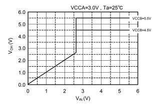
Figure 8 Input/Output Characteristics (Typ.)
