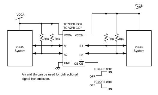
Figure 1 Application Circuit Diagram
