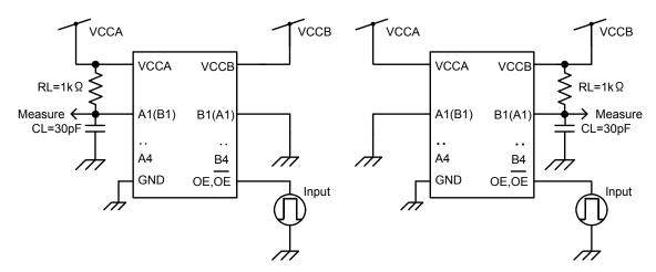
Figure 4 tpLZ, tpZL Test Circuits
