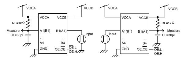
Figure 3 tpLH, tpHL Test Circuits
