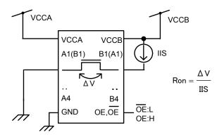
Figure 2 ON-resistance Test Circuits
