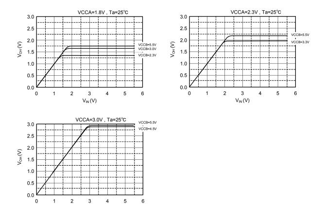
Figure 10 Input/Output Characteristics (Typ.)
