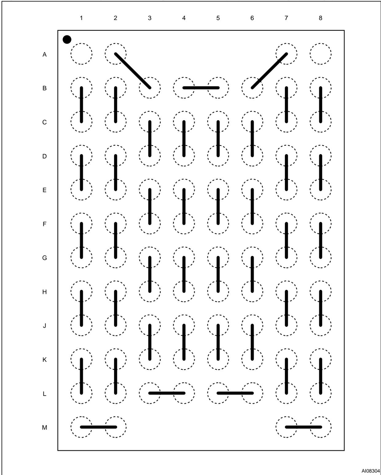
Figure 21. TFBGA88 Daisy Chain - PCB Connection Proposal (Top view through package)
