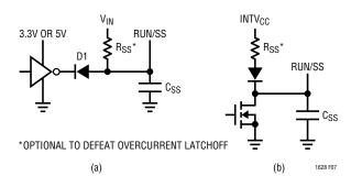
Figure 7. RUN/SS Pin Interfacing
