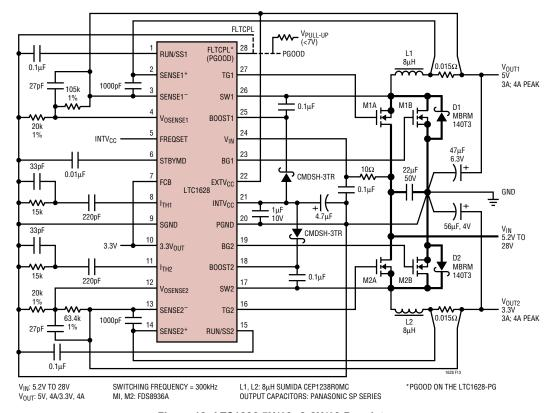
Figure 13. LTC1628 5V/4A, 3.3V/4A Regulator
