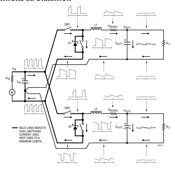
Figure 11. Branch Current Waveforms
