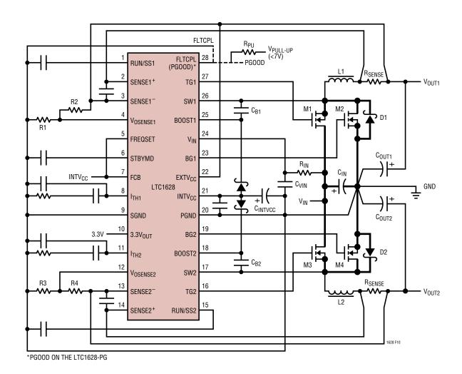
Figure 10. LTC1628 Recommended Printed Circuit Layout Diagram
