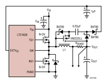
Figure 6b. Capacitive Charge Pump for EXTV<sub>CC</sub>
