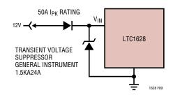
Figure 9. Automotive Application Protection
