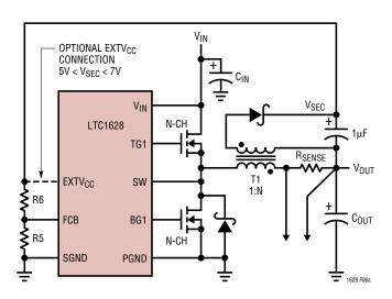
Figure 6a. Secondary Output Loop & EXTV<sub>CC</sub> Connection
