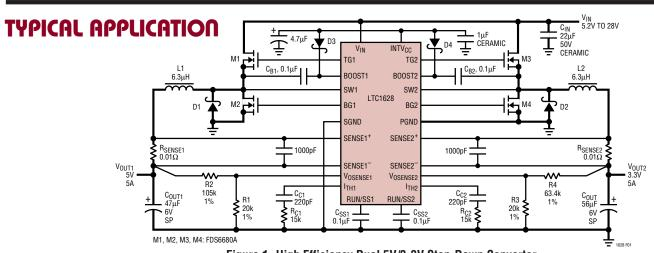
Figure 1. High Efficiency Dual 5V/3.3V Step-Down Converter
