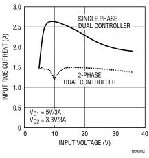
Figure 4. RMS Input Current Comparison
