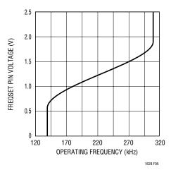
Figure 5. FREQSET Pin Voltage vs Frequency
