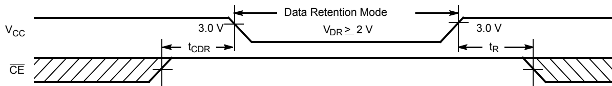
Figure 2. Data Retention Waveform
