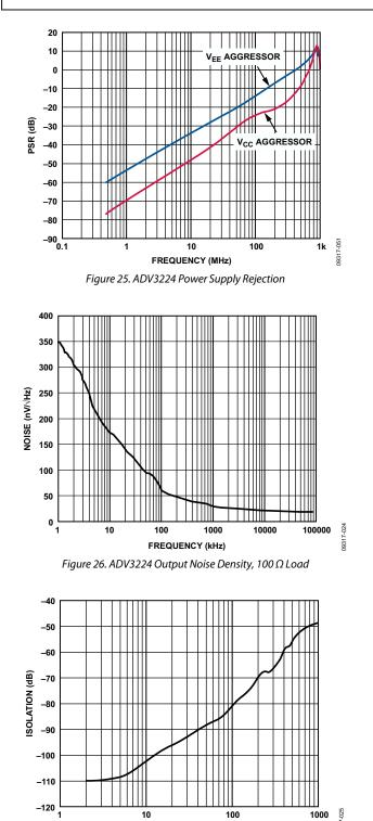
FREQUENCY (MHz) Figure 27. ADV3224 Off Isolation
