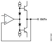
Figure 59. Analog Output Enabled
