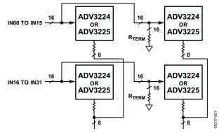
Figure 65. A  $32 \times 16$  Nonblocking Crosspoint Switch Array
