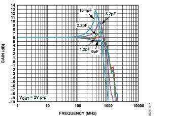
Figure 16. ADV3225 Large Signal Frequency Response with Capacitive Loads
