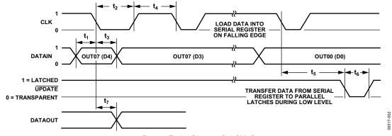
Figure 2. Timing Diagram, Serial Mode
