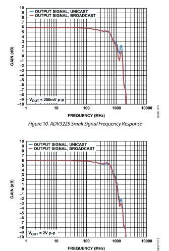
Figure 11. ADV3225 Large Signal Frequency Response
