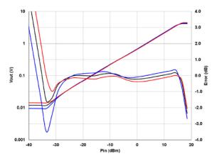
Figure 5 V<sub>OUT</sub> and Conformance Error vs. P<sub>in</sub> and Temperature at 10GHz.
