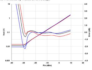
Figure 11  $V_{OUT}$  and Conformance Error vs.  $P_{in}$  and Temperature at 40GHz (Data Truncated by Measurement Setup).
