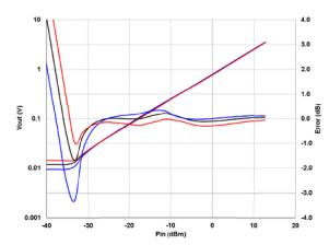
Figure 8  $V_{\text{OUT}}$  and Conformance Error vs.  $P_{\text{in}}$  and Temperature at 25GHz. (Data Truncated by Measurement Setup).
