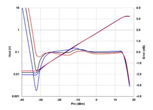
Figure 3 V<sub>OUT</sub> and Conformance Error vs. P<sub>in</sub> and Temperature at 1GHz.
