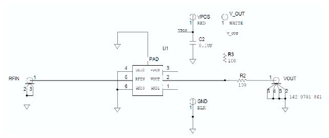
Figure 13 ADL6010 Evaluation Board Schematics
