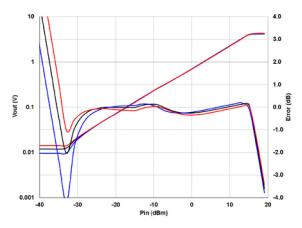
Figure 4 V<sub>OUT</sub> and Conformance Error vs. P<sub>in</sub> and Temperature at 5GHz.
