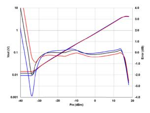
Figure 5 V<sub>OUT</sub> and Conformance Error vs. P<sub>in</sub> and Temperature at 15GHz.
