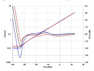
Figure 7  $V_{OUT}$  and Conformance Error vs.  $P_{in}$  and Temperature at 20GHz (Data Truncated by Measurement Setup).
