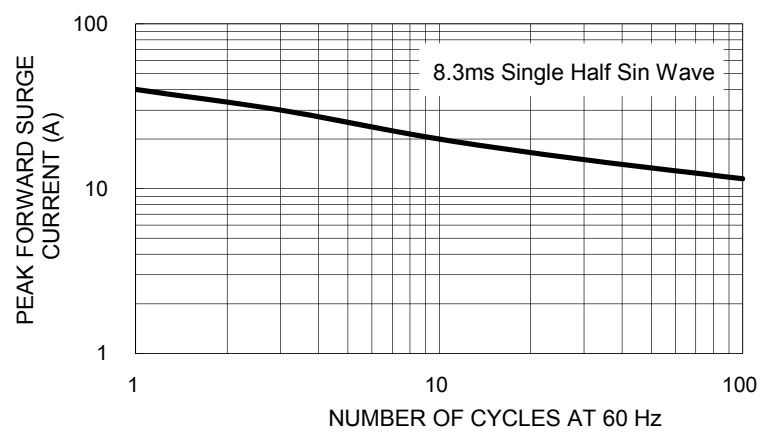
FIG. 2 MAXIMUM NON-REPETITIVE PEAK FORWARD SURGE CURRENT
