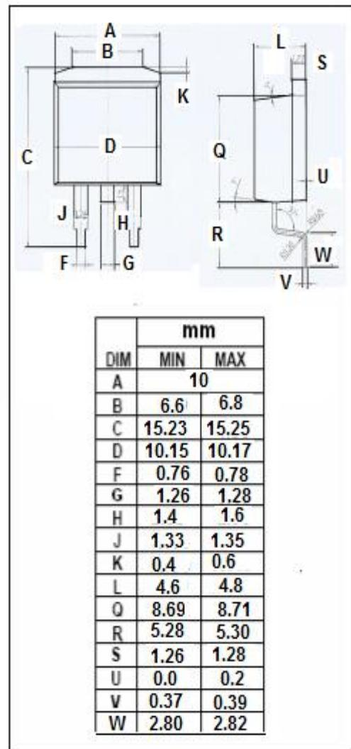
**isc N-Channel MOSFET Transistor**
