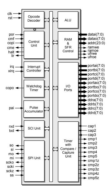
**RAM & SFR Controller** - Data Memory & SFR (Special Function Register) interface controls access into the internal and external program and data memories and special registers. It contains Stack Pointer (SP) register, INIT register (INIT), Data Page Pointer (DPP), Stretch register (ST) and related logic.
