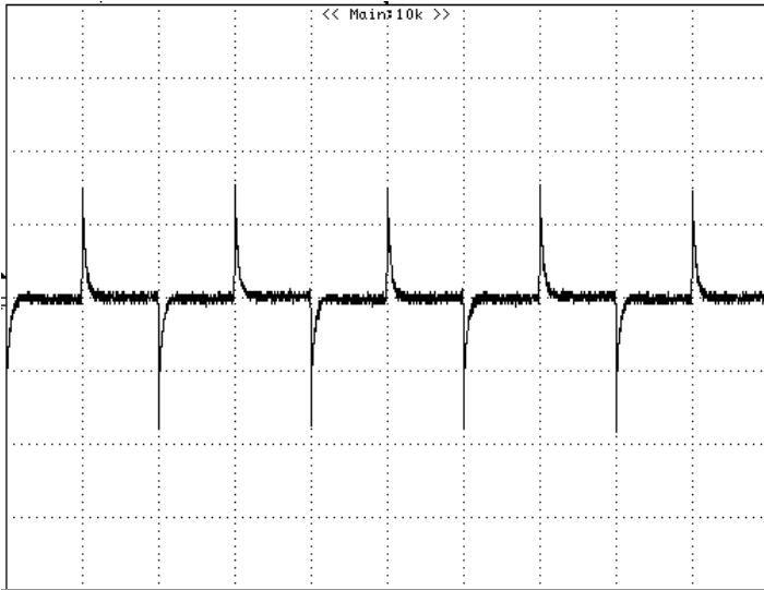
Figure 17: Typical transient response to step load change at 1A/\mu S from 100%~ 0%~100% of I_o , max at 12Vin, 5.0Vout (Cout = 1uF ceramic, 47uF+10uFceramic) CH1 : VOUT, 0.1V/div, 5mS/div
