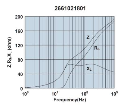
Impedance, reactance, and resistance vs. frequency.
