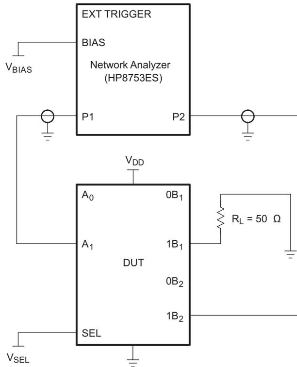
**Figure 8. Test Circuit for Off Isolation ( $O_{IRR}$ )**
