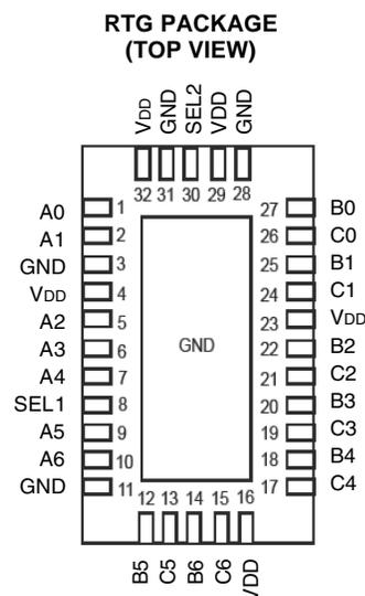
The exposed center pad must be connected to GND.
