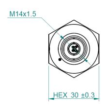
All dimensions are millimeters (mm). Mating connector type is FCI female receptacle ref. 54200409 (black-sealed). Sensor body is stainless steel. M14 Viton O'ring provided for hermetical mounting.
