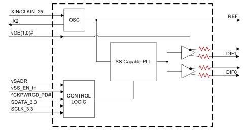
Note: Resistors default to internal on 41/51 devices. P1 devices have programmable default impedances on an output-by-output basis.
