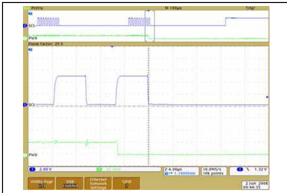
FIGURE 2-53: 100 k \Omega – Low-Voltage Decrement Wiper Settling Time ( V_{DD} = 5.5\text{V} ) (1 \mu\text{s}/\text{Div} ).
