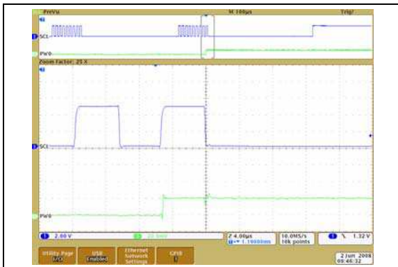
FIGURE 2-55: 100 k \Omega – Low-Voltage Increment Wiper Settling Time ( V_{DD} = 5.5\text{V} ) (1 \mu\text{s}/\text{Div} ).
