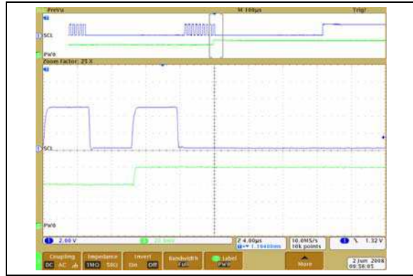
FIGURE 2-17: 5\text{ k}\Omega – Low-Voltage Increment Wiper Settling Time ( V_{DD} = 5.5\text{V} ) ( 1\text{ }\mu\text{s/Div} ).
