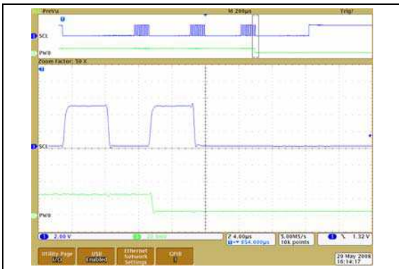
FIGURE 2-41: 50 k \Omega – Low-Voltage Decrement Wiper Settling Time ( V_{DD} = 2.7\text{V} ) (1 \mu\text{s}/\text{Div} ).
