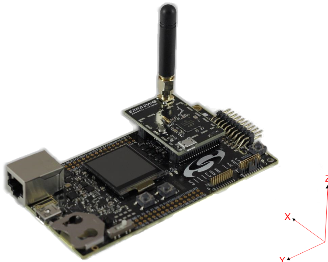
Figure 6.2. DUT: BRD4503B (Rev. A00) Radio Board with Wireless Starter Kit Mainboard
