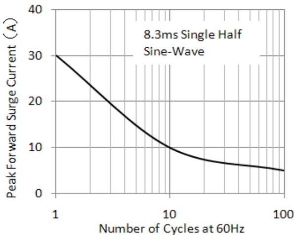
Figure 5. Maximum Non-Repetitive Peak Forward Surge Current
