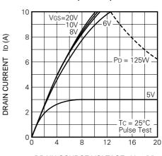
DRAIN-SOURCE VOLTAGE VDS (V)
