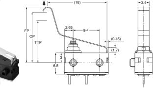
Note1. Unless otherwise specified, a tolerance of ±0.2 mm applies to all dimensions. Note2. The operating characteristics are for operation in the A direction ( $\clubsuit$ ).
