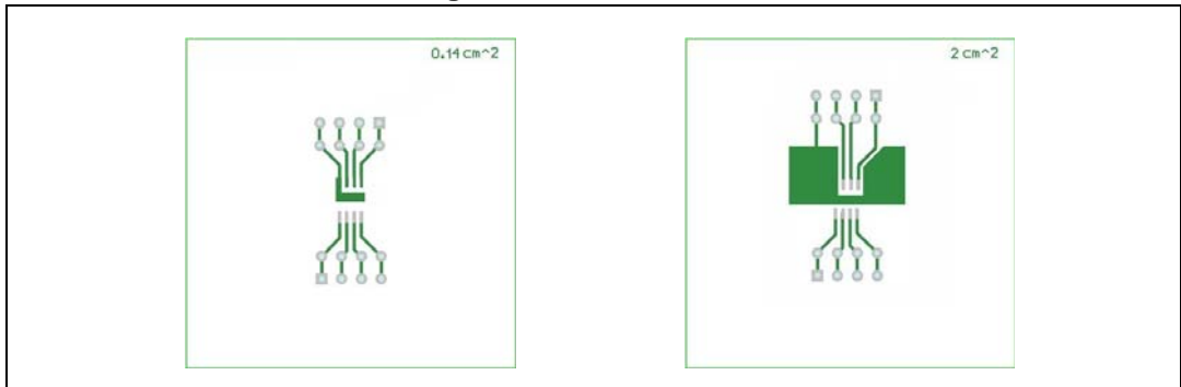
Figure 23. SO-8 PC board
