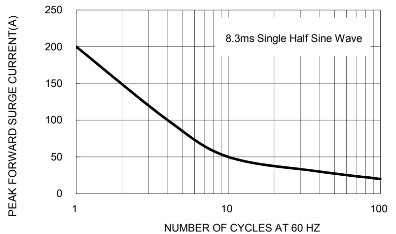
FIG. 2 MAXIMUM NON-REPETITIVE PEAK FORWARD SURGE CURRENT
