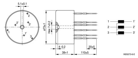
Dimensions in mm Tolerances acc. ISO 2768-c
