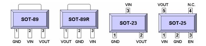
Figure 2: Pin Configuration
