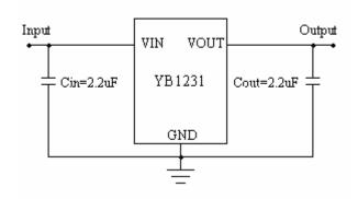
Figure 1-2: SOT-23/SOT-89 Application Circuit
