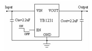
Figure 1-1: SOT-25 Application Circuit
