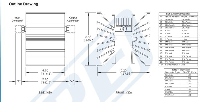
20 dB Fixed Attenuator, SMA Female To SMA Female Directional Black Aluminum Heatsink Body Rated To 300 Watts Up To 3 GHz from Pasternack Enterprises has same day shipment for domestic and International orders. Our RF, microwave and millimeter wave products maintain a 99% availability and are part of the broadest selection in the industry.
