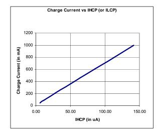
Using the table below it can be seen that for a programming current value of  $11.4\mu A$ , the corresponding maximum charge current is 92mA.
