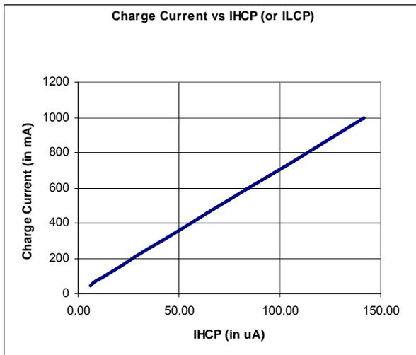
Using the table below it can be seen that for a programming current value of 11.4µA, the corresponding maximum charge current is 92mA.
