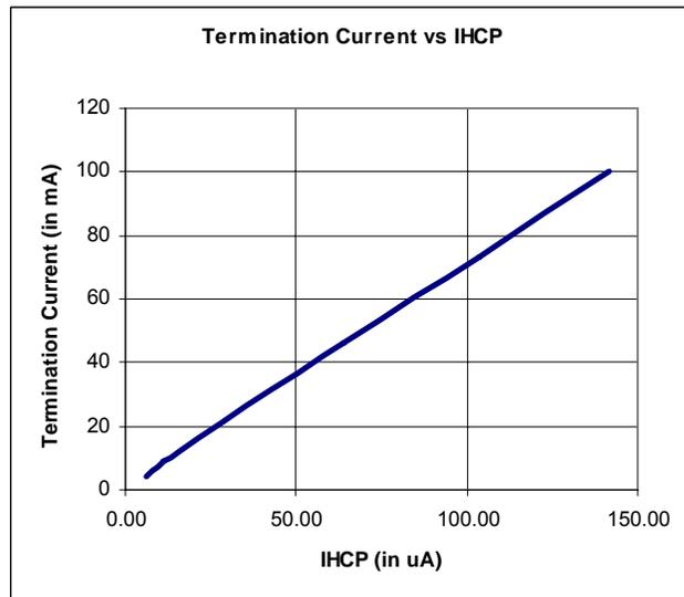
The termination current is always roughly 10% of the maximum charge current set by the HCP resistor.
