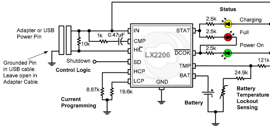
**Figure 1** – Typical Application – 1A or 500mA maximum charge currents with three indicators and battery temperature lockout. A grounded spare pin in the USB power cable can be used to sense when the 500mA USB current power source is being used.
