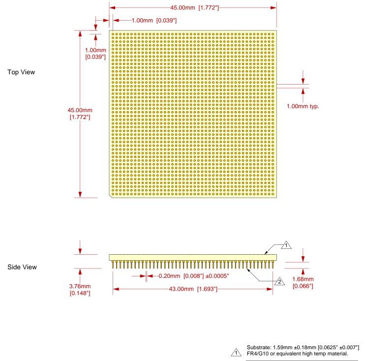
Pins: material- Brass Alloy 360 1/2 hard; finish-0.25μm [10μ"] Au over 1.27μm [50μ"] Ni (min.).
