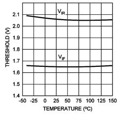
Figure 10. Input Thresholds vs Temperature
