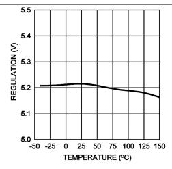
Figure 15. HB Regulation Voltage vs Temperature
