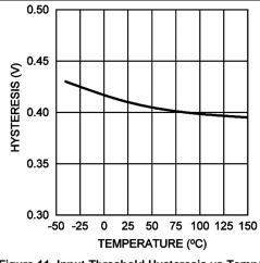
Figure 11. Input Threshold Hysteresis vs Temperature
