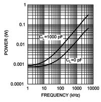
Gate-driver power dissipation (LO+HO), VDD = +5 V
