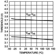
Figure 9. UVLO Falling Thresholds vs Temperature
