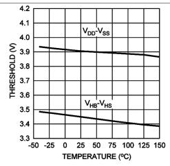
Figure 8. UVLO Rising Thresholds vs Temperature
