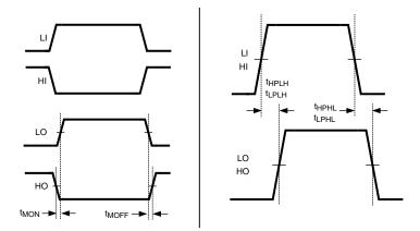
Figure 1. Timing Diagram
