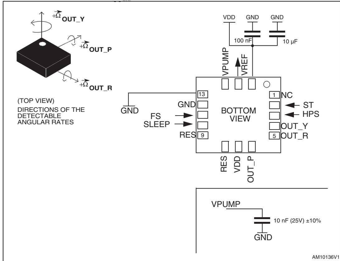
Note: The capacitor on pin 14 must guarantee a 1 nF value under 11 V bias condition.
