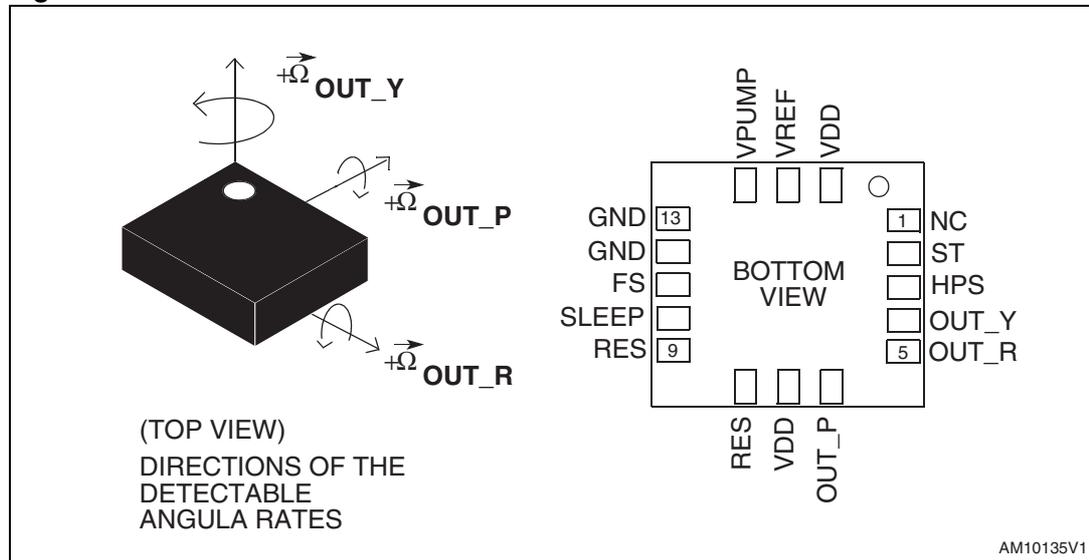
Note: The vibration of the structure is maintained by drive circuitry in a feedback loop. The sensing signal is filtered and appears as an analog output.
