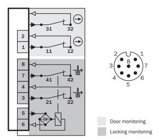
$\ensuremath{\mbox{\fontfamily}}$  Positive action N/C locking monitoring contact
