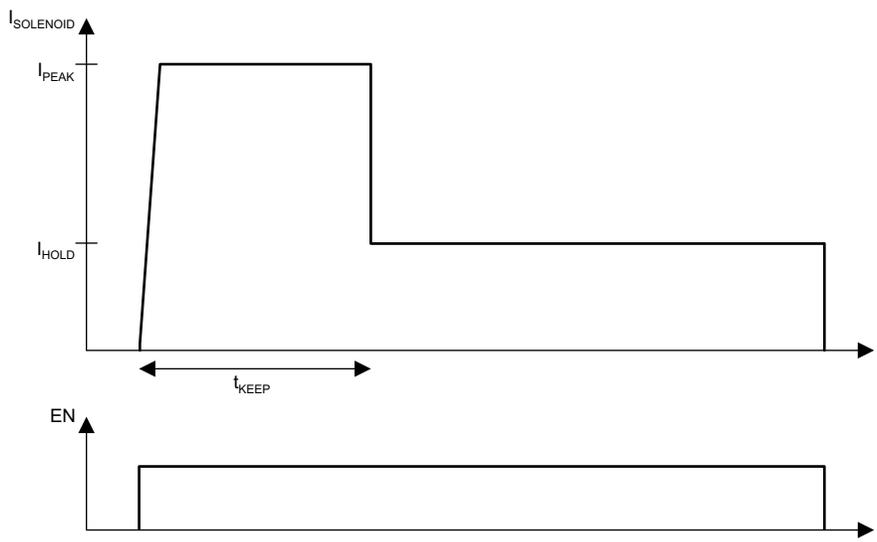
**Figure 2. Typical Current Waveform Through the Solenoid**
