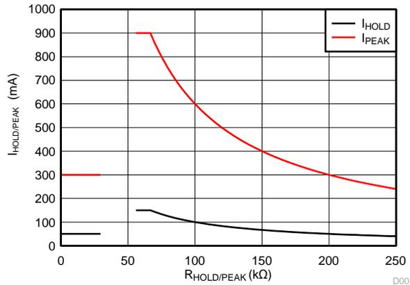
**Figure 4. I<sub>PEAK</sub> and I<sub>HOLD</sub> settings for R<sub>SENSE</sub> = 1 Ω**
