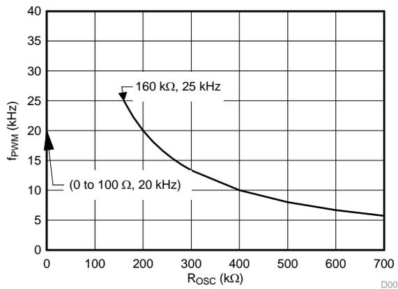
**Figure 5. PWM Clock Frequency Setting**
