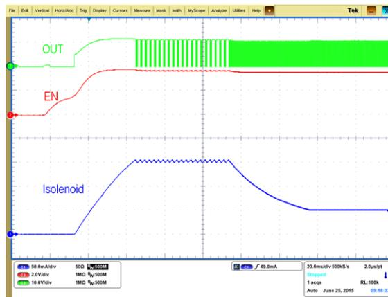
Figure 1. Solenoid Current, EN, and PWM vs Time
