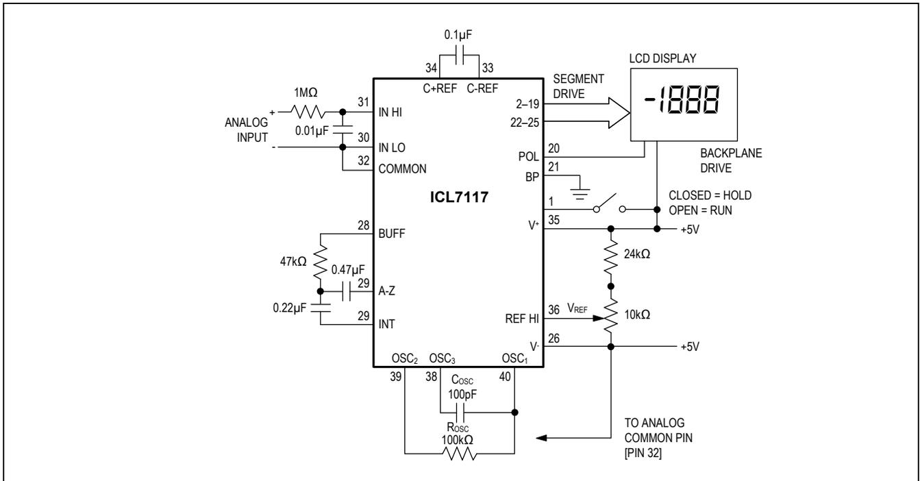
Figure 2. Maxim ICL7117 Typical Operating Circuit, 200mV Reference
