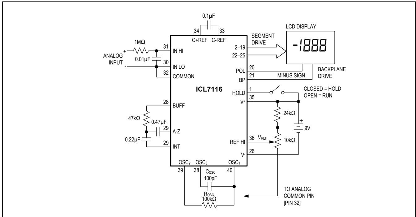
Figure 1. Maxim ICL7116 Typical Operating Circuit, 200mV Reference
