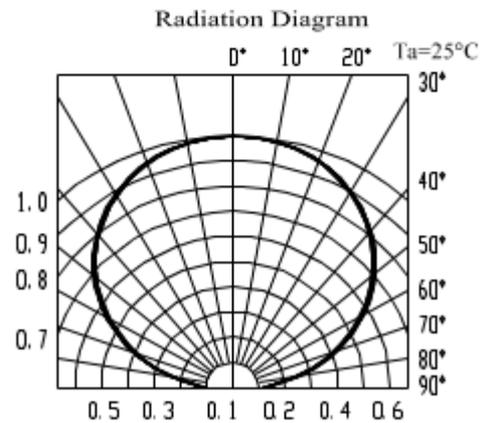
**Typical Electro-Optical Characteristics Curves
