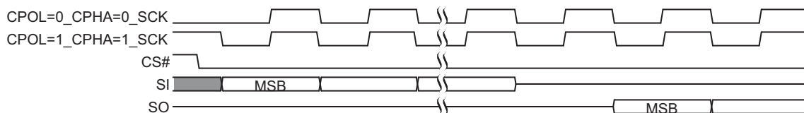
Figure 3.1 SPI SDR Modes Supported
