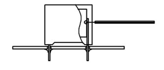
Temperature monitored inside the capacitor.
