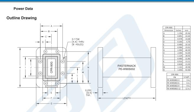
WR-90 Commercial Grade Straight Waveguide Section 3 Inch Length with CPR-90G Flange Operating from 8.2 GHz to 12.4 GHz from Pasternack Enterprises has same day shipment for domestic and International orders. Our RF, microwave and millimeter wave products maintain a 99% availability and are part of the broadest selection in the industry.
