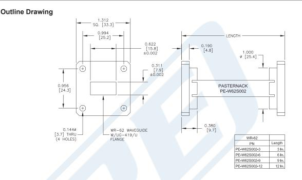
WR-62 Instrumentation Grade Straight Waveguide Section 6 Inch Length with UG-419/U Flange Operating from 12.4 GHz to 18 GHz from Pasternack Enterprises has same day shipment for domestic and International orders. Our RF, microwave and millimeter wave products maintain a 99% availability and are part of the broadest selection in the industry.
