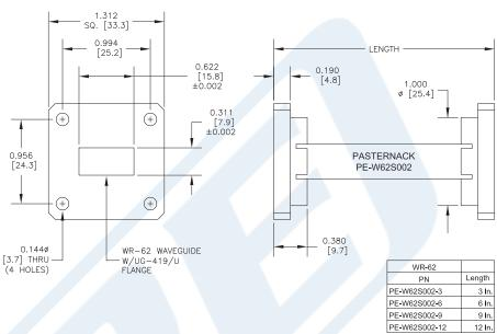
WR-62 Instrumentation Grade Straight Waveguide Section 3 Inch Length with UG-419/U Flange Operating from 12.4 GHz to 18 GHz from Pasternack Enterprises has same day shipment for domestic and International orders. Our RF, microwave and millimeter wave products maintain a 99% availability and are part of the broadest selection in the industry.
