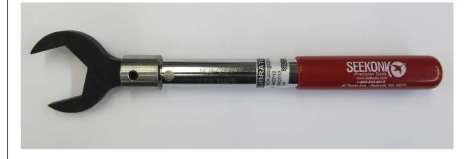
Pre-set at factory to desired value within a +/- 4% tolerance. When preset torque value is achieved, a distinct click is felt and heard, followed by a sudden release into several degrees of free movement. Ideal for applications in which one torque value is used extensively. Compact design makes these tools invaluable in hard to reach locations. Tools automatically reset when torquing- force is removed.
