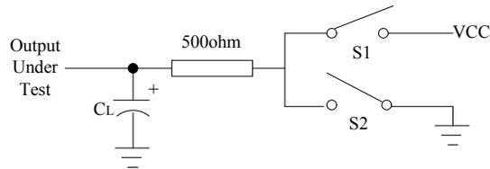
Figure 6. Driver Enable and Disable Timing Test Load
