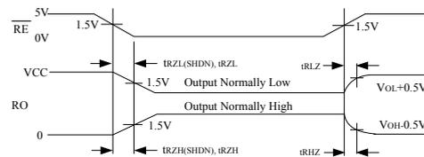
Figure 10. Receiver Enable and Disable Times
