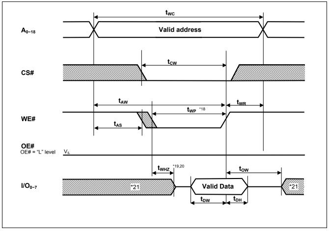
Note 18.  $t_{WP}$  is the interval between write start and write end.
