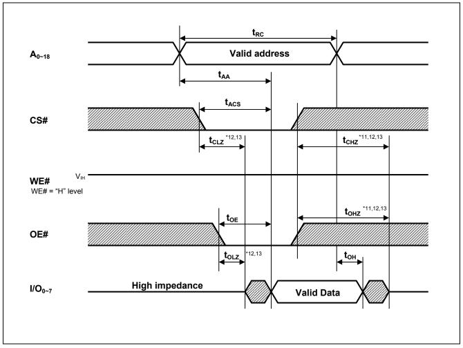
Note 11.  $t_{CHZ}$  and  $t_{OHZ}$  are defined as the time when the I/O pins enter a high-impedance state and are not referred to the I/O levels.
