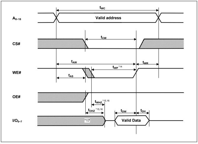
Note 14.  $t_{WP}$  is the interval between write start and write end.
