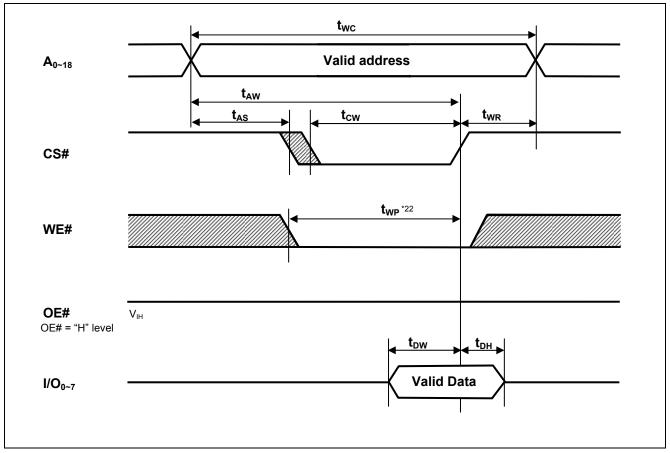
Note  $\,$  22.  $\,$   $t_{WP}$  is the interval between write start and write end.
