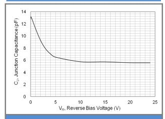
Fig.1 Typical Junction Capacitance(24V)
