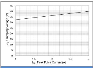
Fig.3 Typical Peak Clamping Voltage(8/20µs)(24V)
