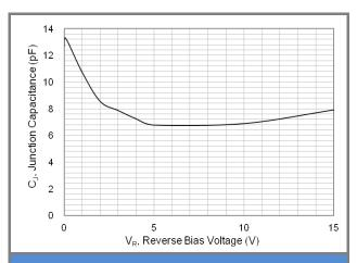
Fig.2 Typical Junction Capacitance(15V)
