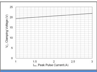
Fig.4 Typical Peak Clamping Voltage(8/20μs)(15V)
