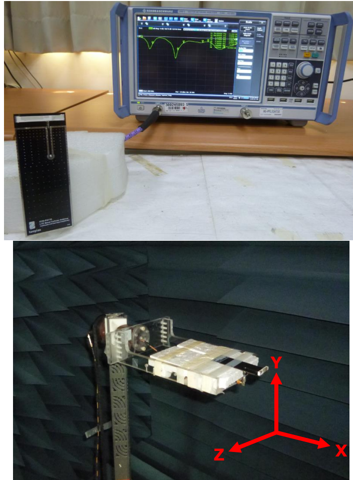
Figure 1. Impedance measurements (left hand) and peak gain, average gain, efficiency and radiation pattern measurements (right hand)
