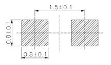
**Notes:** 1.All dimensions are in millimeters 2.Tolerances unless dimensions ±0.1mm
