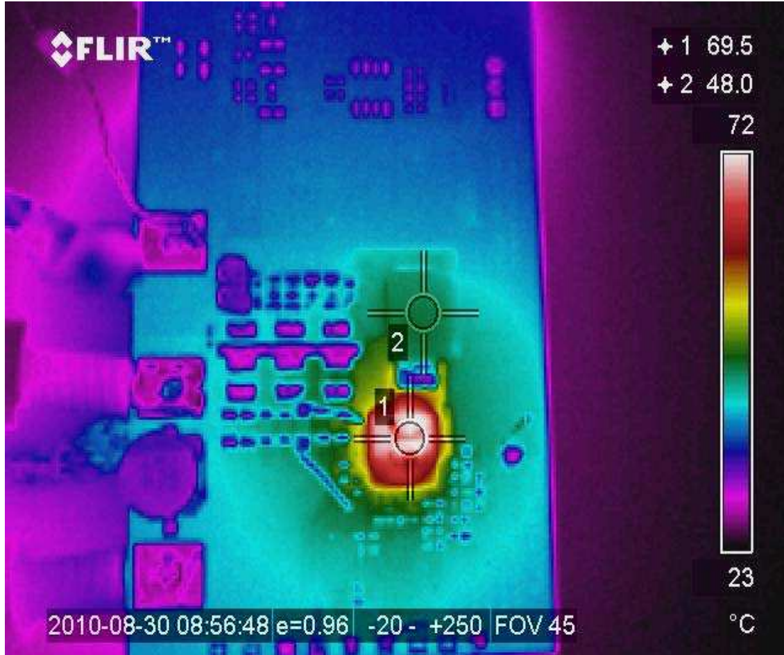
Figure 31: Thermal Image of the board at 35A load Test point 1 is iP1837 Test point 2 is inductor
